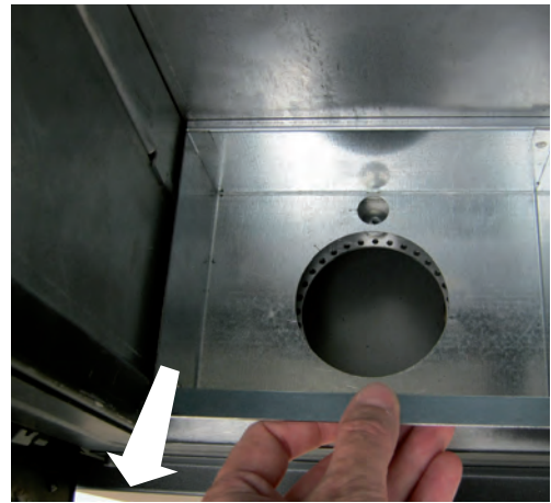
Fig. 14: cleaning the ash box
