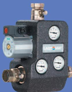
With its design, Laddomat 21 substitutes classical installation principle based on single components. Its consists of a cast-iron body, thermo-regulation valve, pump, non-returning valve, ball valves and thermometers. When water in the boiler reaches 78 °C (72 °C), the thermo-regulation valve opens supply from the return pipeline. Installation with the Laddomat 21 is much simpler and therefore we can highly recommend it.
