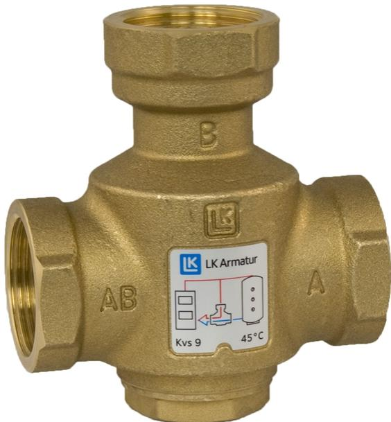
LK 823 ThermoVar® is a 3-way thermic loading valve for solid fuel/storage tank installations. The valve is intended to ensure both an optimal temperature stratification in the storage tank and a high return temperature to the boiler, thus increasing the efficiency of the system. Tarring and condensation are prevented which prolongs boiler life.
